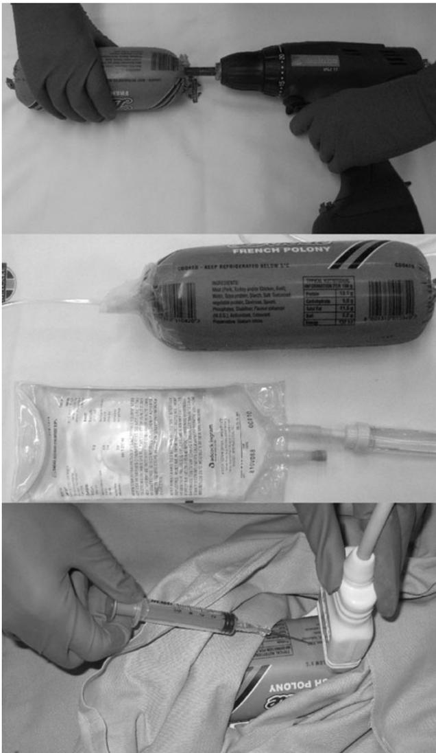
**Fig. 1** The construction of the central venous access polony phantom. First a hole is carefully bored from one end of the polony with a low-speed drill, then an expired IV is connected to keep the vein filled. Standard techniques can be used for the simulated vascular access
