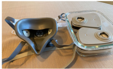
1. Inspect the mask and filter for damage, paying attention to the inner gaskets and valves.
